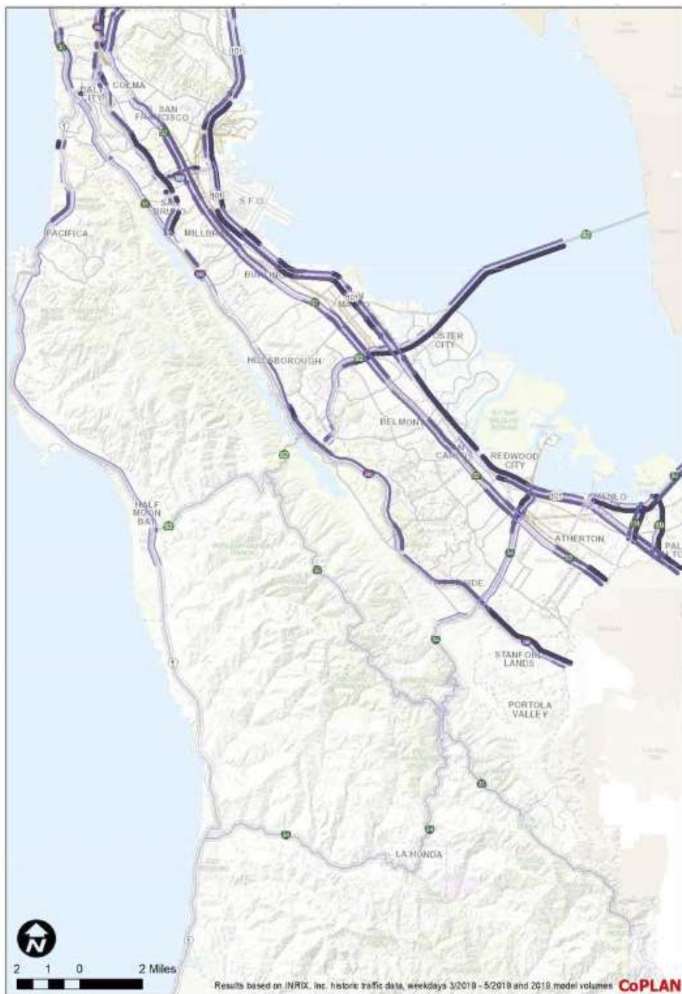
Legend VHD/Mile — 0 - 25 — 26 - 50 — 51 - 75 — 76 - 150 — 151+ Source: State Highway System Congestion and Safety Assessment Update 2019 Figure 3-2. Total Vehicle Hours of Delay Per Mile - Evening Peak Hour
